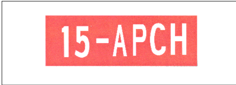
FIG 2-3-27 Holding Position Sign for a Runway Approach Area
