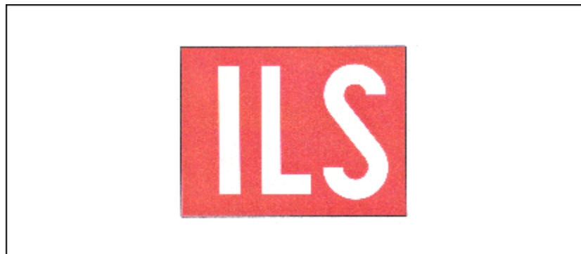
FIG 2-3-28 Holding Position Sign for ILS Critical Area
