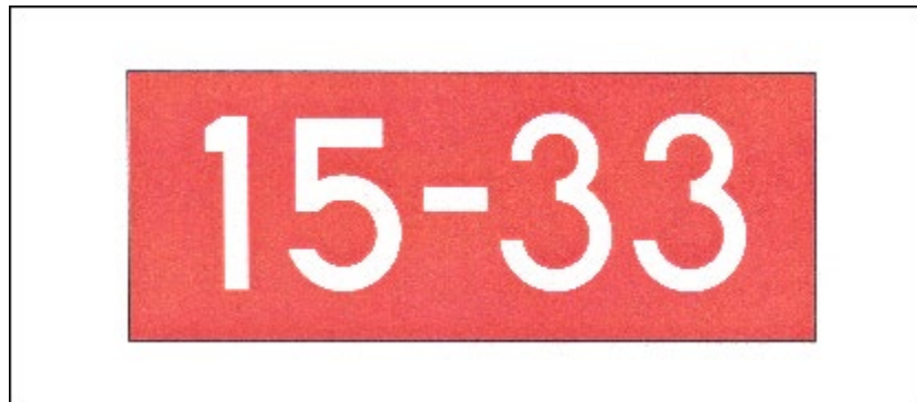
FIG 2-3-24 Runway Holding Position Sign
