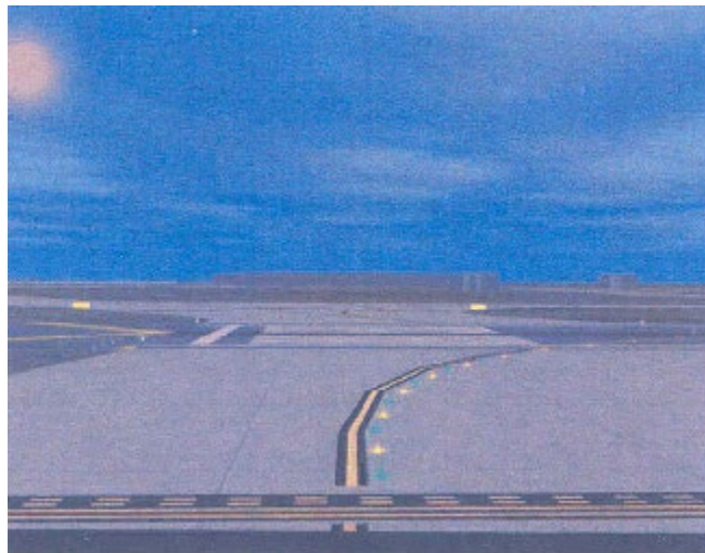
FIG 2-1-14 Taxiway Lead-On Light Configuration
