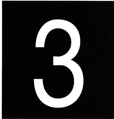
FIG 2-3-41 Runway Distance Remaining Sign Indicating 3,000 feet of Runway Remaining
