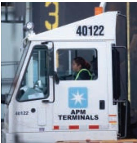
**The yard hostler prototype at APM Terminal will be the heaviest gross-weight application of hydraulic hybrid technology to date.**
