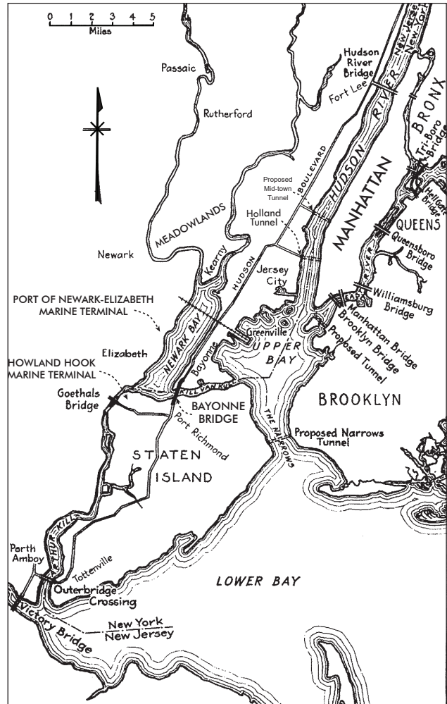
This map shows the bridges, tunnels, and proposed tunnels that were designed to link together the network of roadways between New York and New Jersey in 1931. While some of the proposed links were never constructed, the map illustrates the complex system that the Bayonne Bridge was and is a part of.
