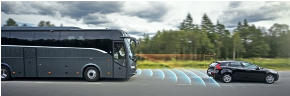
Figure 14: Forward Collision Warning
