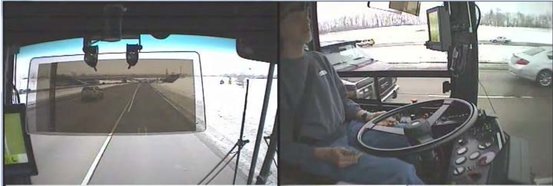
Figure 13: Screen Capture from video from MTVA Driver-Assist System Showing Heads-Up Display and Autonomous Steering for Lane Keeping
