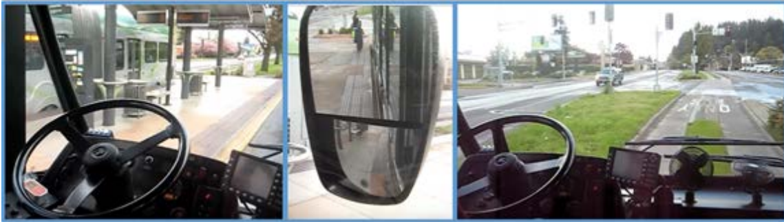
Figure 6: Example of Automated Steering and Precision Docking from Lane Transit District
