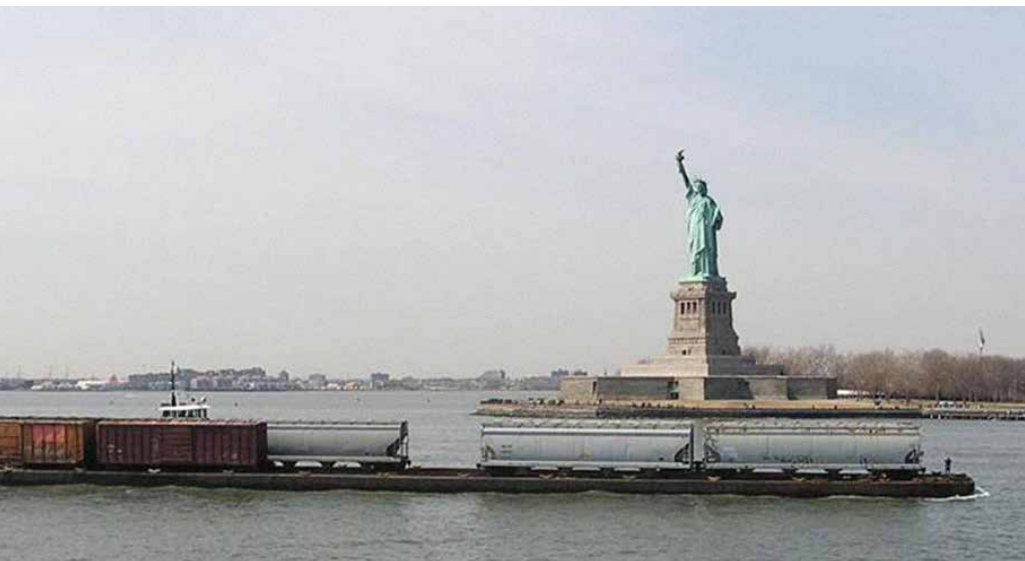
New York New Jersey Rail, LLC railcar float allows for cross-harbor rail freight movement, an alternative to the use of regional highways.
