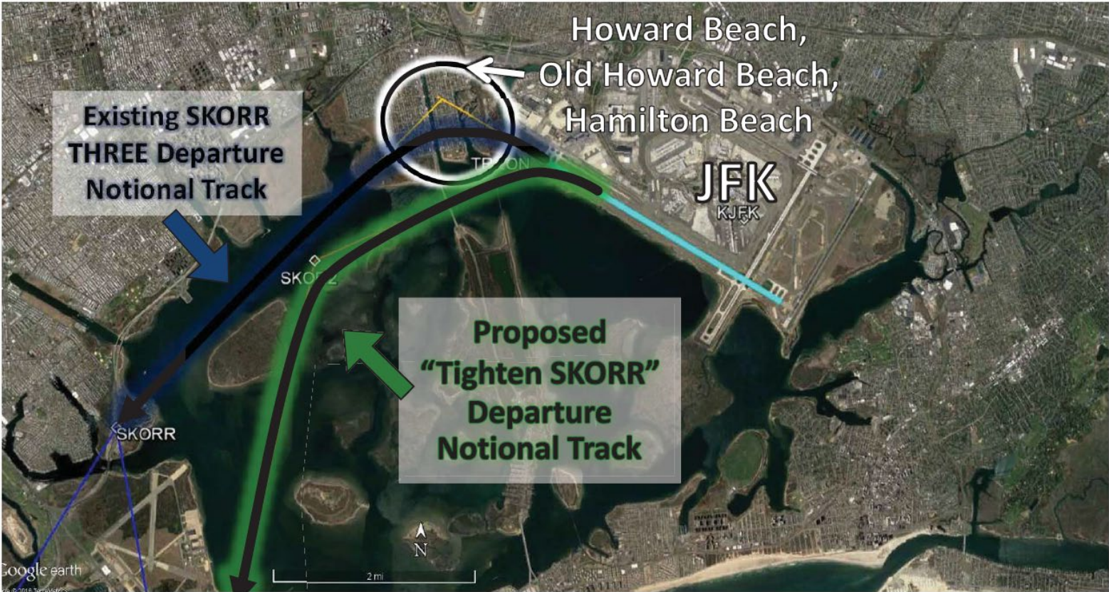
Figure 2-2 Existing SKORR THREE and Proposed "Tighten SKORR" Notional Tracks - Example for Runway 31L John F. Kennedy International Airport
