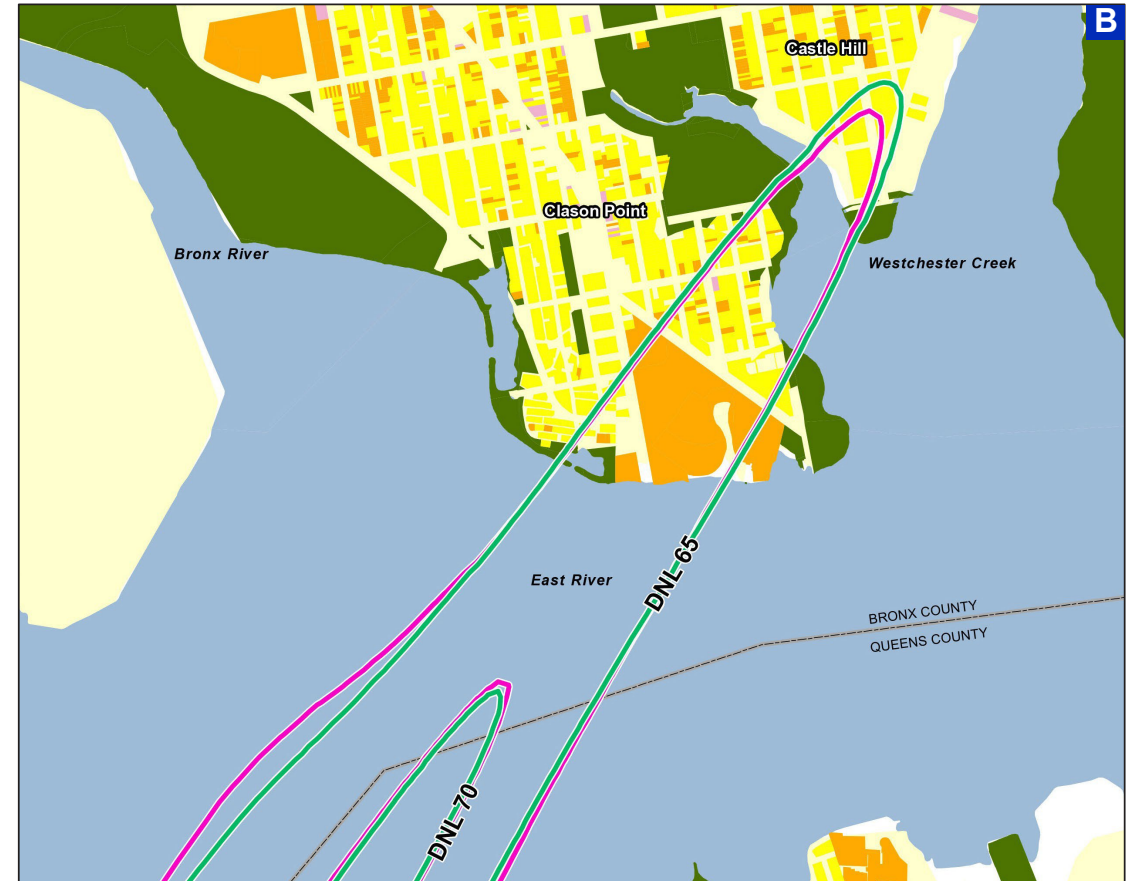
NADP1 and NADP2 DNL 65, 70, and 75 Contours over Clason Point and Castle Hill
