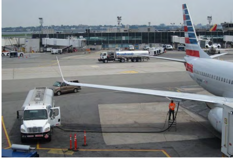
Figure 22: Bowser Fueling Operation
