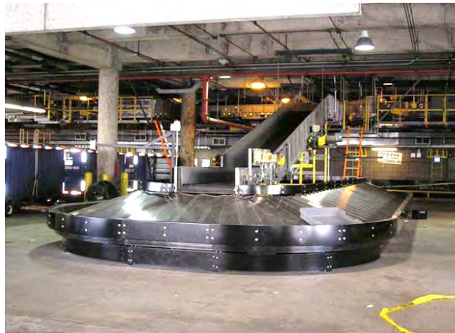
Figure 32: Sloped-Plate Bag Make-up Device 26
