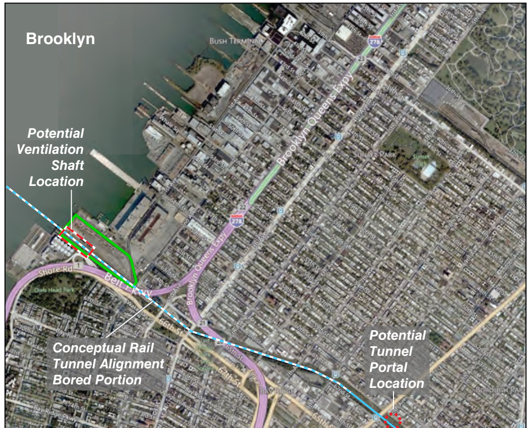
FIGURE 4-15 Potential Tunnel Portal and Ventilation Shaft Locations CROSS HARBOR FREIGHT PROGRAM
