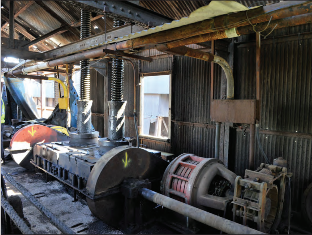
Lift Bridge Motors in Situ
